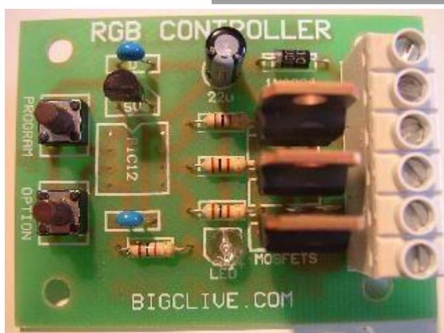
Then install the MOSFETs into the PCB as shown.
