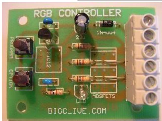
Two components are fitted in this picture. The 22uF electrolytic capacitor and the terminal block. The capacitor absolutely **MUST** be inserted the correct way round. Again the longest lead is the positive connection and a grey band on the case indicates the negative side. Double check the pictures to make sure you have it in the right way round. It's function is to smooth out any dips or transients in the main supply to provide the control circuitry with steady power.
