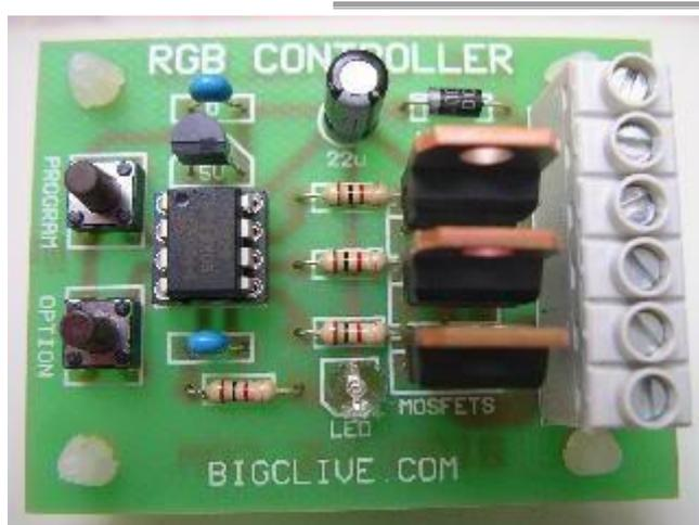
Finally fit the control chip. This probably came already clipped into it's socket, but if you like you can carefully remove the chip from the socket by carefully prising it out from both sides with a thin screwdriver. On the other hand you can just solder the whole assembly in as supplied. (Which is easier.)
