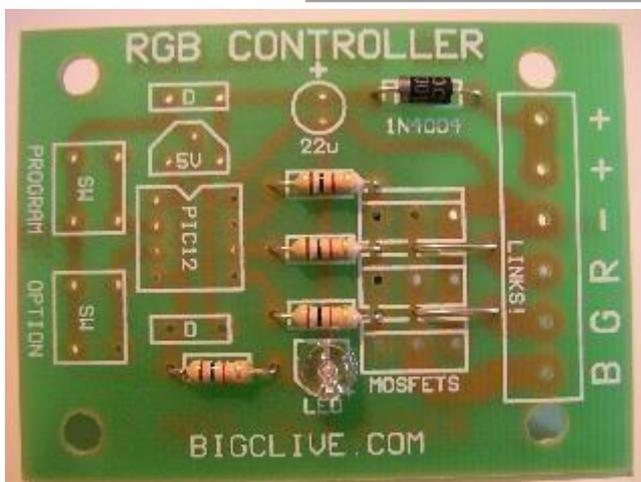
Next is the power indicator LED. This indicates when the circuitry has power and will only work if it's installed the correct way round. The longest lead is the anode and goes to the hole nearest the "+" symbol.
