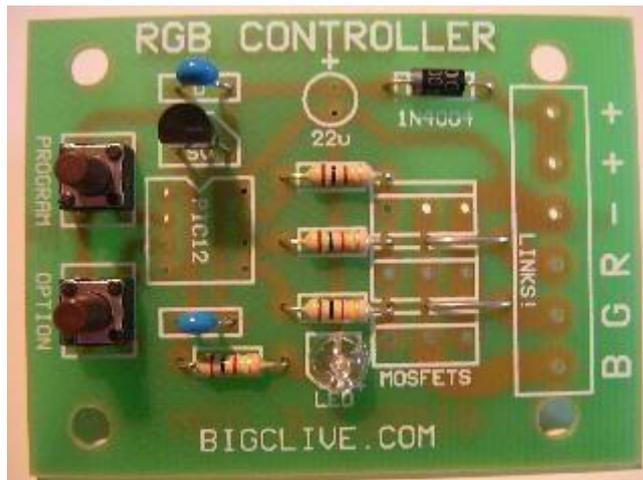
Now fit the little three pin voltage regulator making sure that it's the correct way round as shown above.
