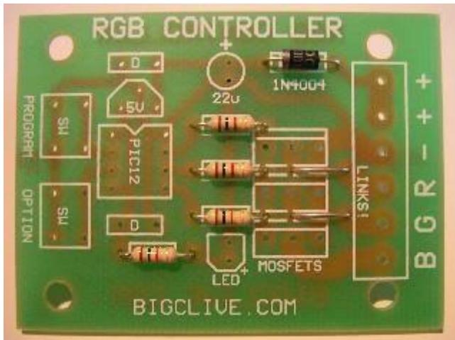
Next fit the diode. This is a common 1A rectifier diode and is used to protect the circuitry from wrong connection of the supply. It only allows current to flow in one direction, so must be fitted the right way round.
