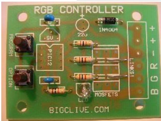
Next are the two push button switches. These are designed to push-fit into the PCB and are very easy to solder.
