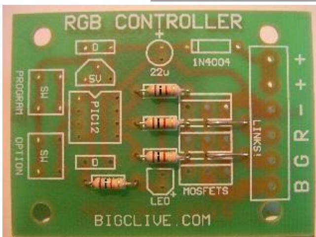
It's a good idea to fit the components in order of size, so fit the resistors next. These
