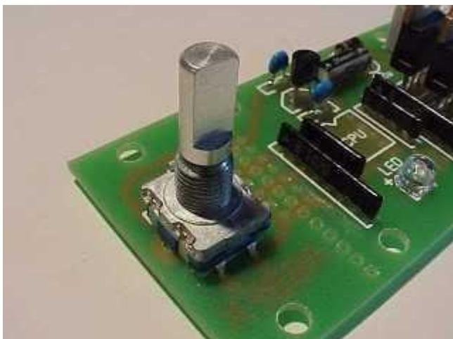
Be extra careful in mounting and soldering the rotary encoder. This is a fairly high resolution gray code unit and has a lot of small contacts inside it. Once you've carefully jiggled the large support pins and the five small connector pins into the PCB, solder the big support pads first, then carefully solder the five other pins without lingering on them with the soldering iron for too long.
