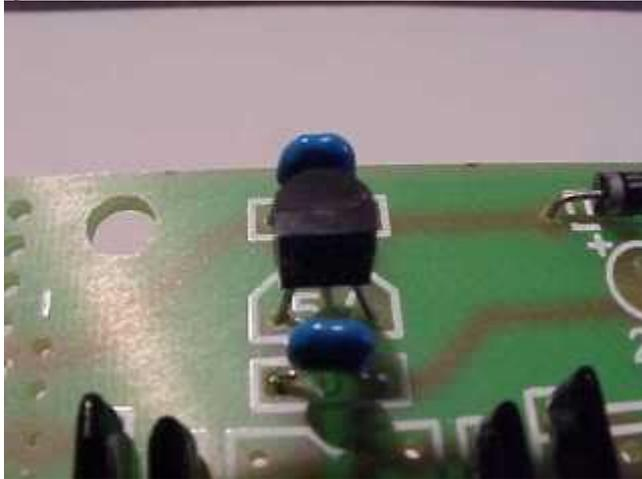
Now we fit the little three pin voltage regulator (78L05) which goes into the position marked 5V as shown.
