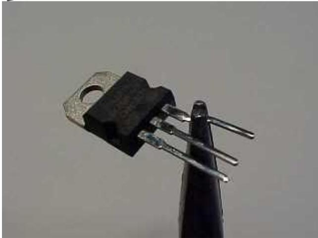
The MOSFETs will need their outer leads bent slightly to make them fit in the PCB holes. This was done to allow much bigger pads and tracks to be used.
