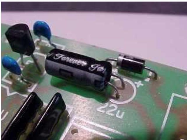
You have a choice in mounting the electrolytic capacitor. You can either leave it standing up on the PCB or lay it down flat. As you can see, I chose the latter. Make sure that the longer lead goes to the side marked with plus symbols. The negative stripe printed on one side should face away from the diode as shown. If you fit that component in the wrong way round it might go POP!
