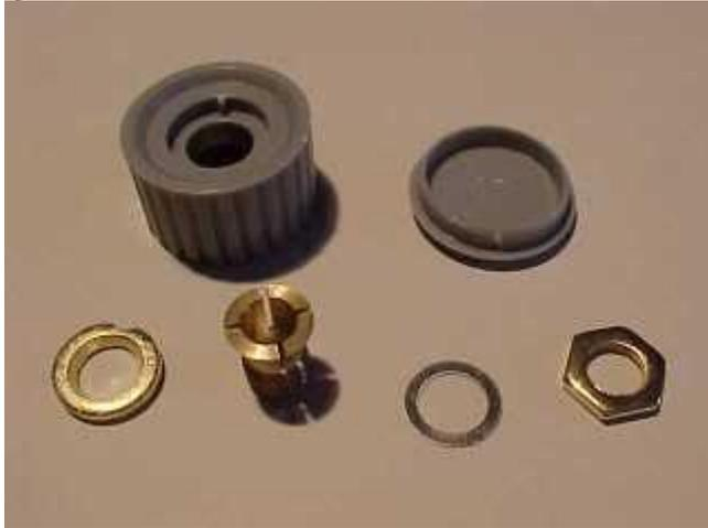
The knob itself has six components! Apart from the grey plastic knob and lid there are four metal components as follows.
