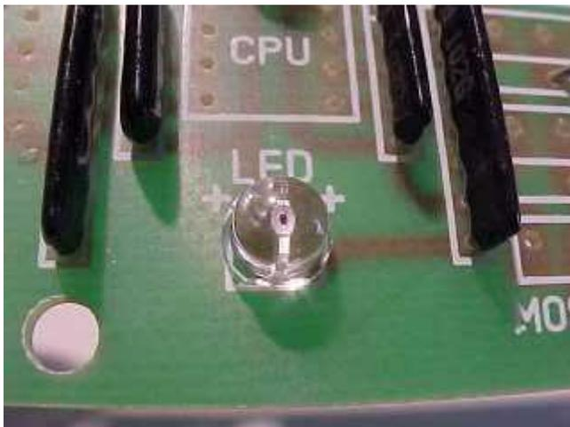
Next is the power indicator LED. This indicates when the circuitry has power and will only work if it's installed the correct way round. The longest lead is the anode and goes to the hole nearest the "+" symbols.
