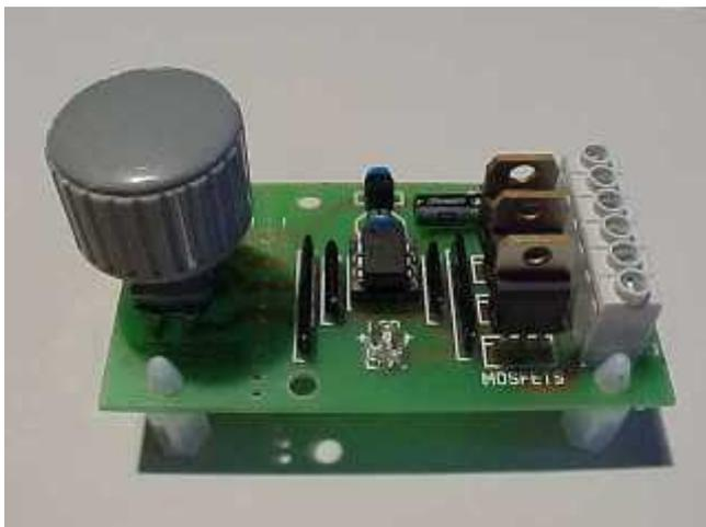
Finish the controller by adding the knob to the encoder and the four support feet. There are six holes for the support feet to allow for whether the knob is on board or mounted remotely.
